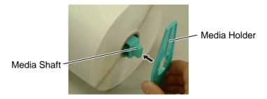
**7.** Insert the Media Holder Ass'y into the slots of the printer.
